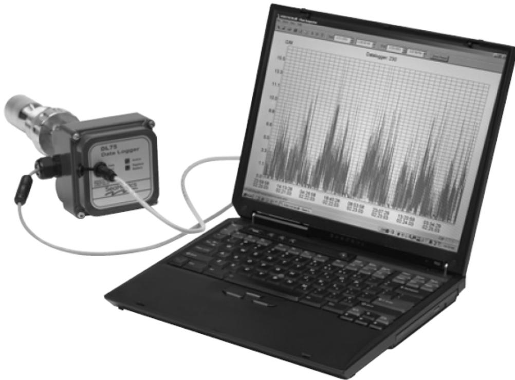
**1. Seametrics turbine-style flow meter with logger and computer.**
